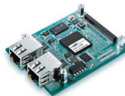
Integration module with PROFINET Device Stack or Controller Stack
